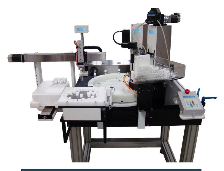
Shown with options: Bulk tube load magazine, cap feeder, programmable XY tray packaging.
