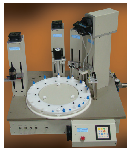
Complete system for filling, tipping, capping and more in a truly space saving benchtop design.
